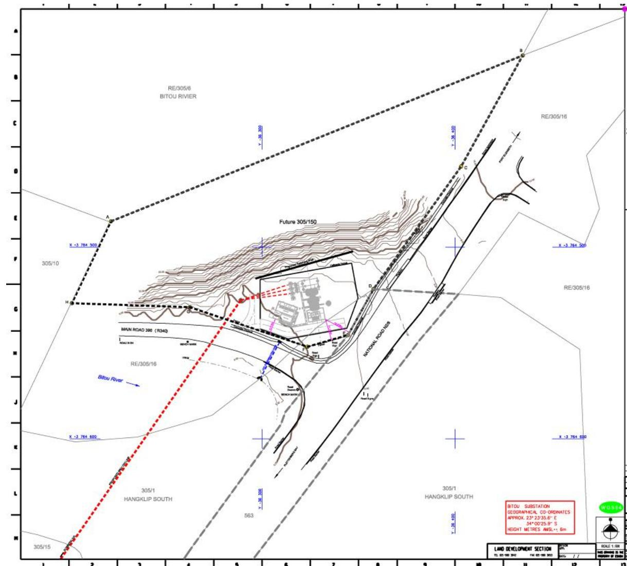
**Figure 1. Site plan for the proposed development. Red dashed lines indicate the proposed power line. (Source: Eskom).**
