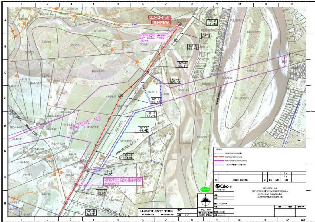
Figure 2. Site plan showing the wider area and the direction of the proposed power lines (dotted red line) and supportive pylons (concentric black rings).
